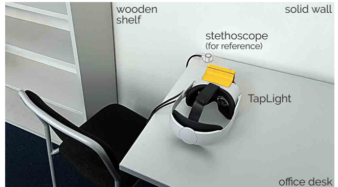
Figure 6: In our technical evaluation, participants provided touch events on these three surfaces. To evaluate TapLight’s depth accuracy, the headset was additionally equipped with retroreflective Optitrack markers.
